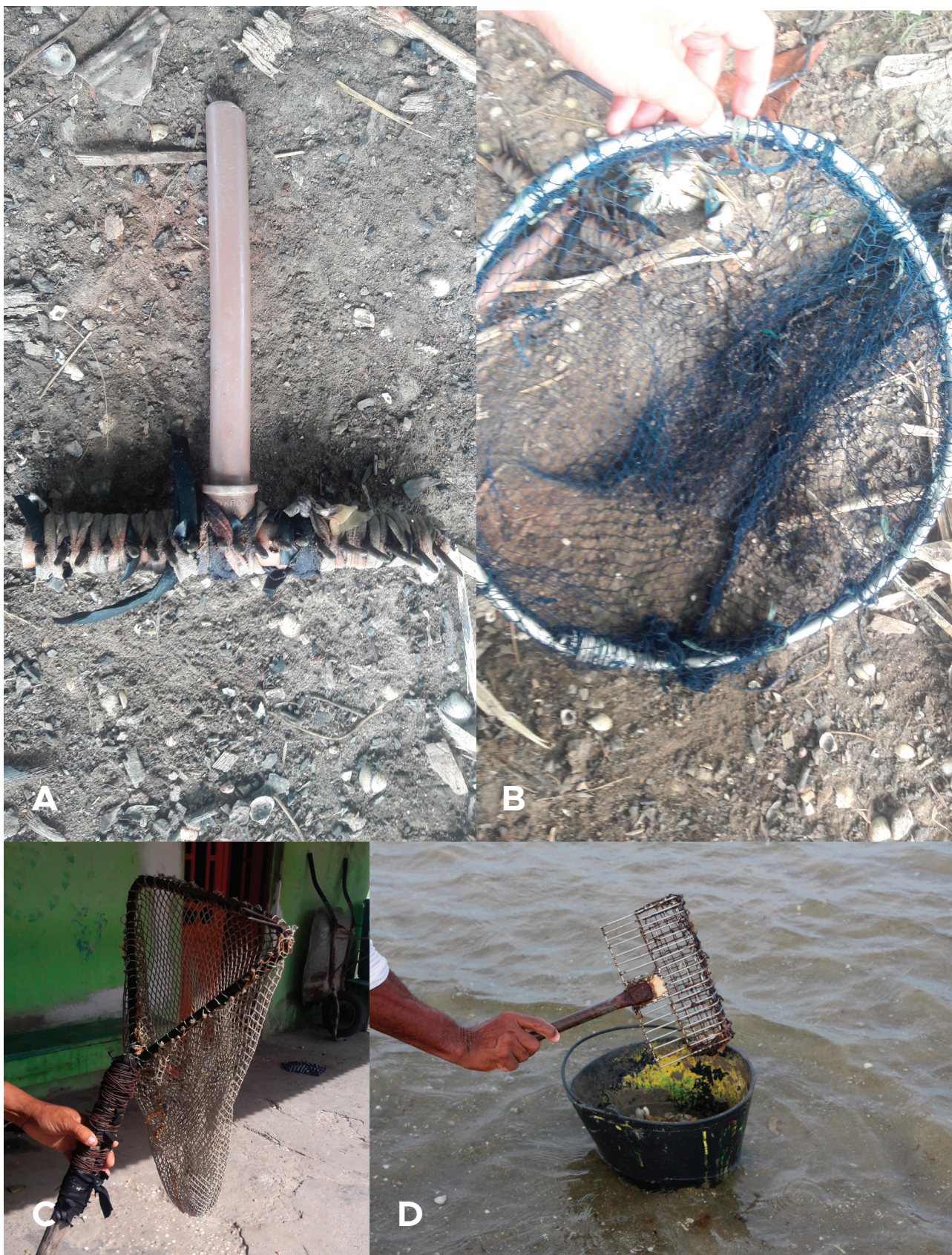
Figure 3. Fishing equipment used to enhance the catching capacity of the Anomalocardia flexuosa (LINNAEUS, 1767). A) Gadanho. B), C), and D) Puça variations. Source: Ivo Raposo, 2017/2018.
